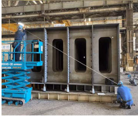
(a) Fabrication of reaction beam
