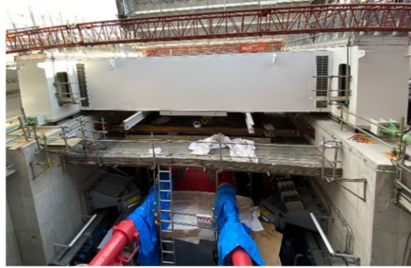
(b) Installed reaction beam on elastomeric isolator bearings
